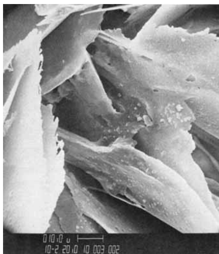
Fig. 1. SEM of powdery class-I poly(glycidyl methacrylate) coating on aluminum cathode obtained by electrolysis of 0.440M glycidyl methacrylate-0.030M sodium acetate-dichloromethane solution at 5 volts for 17 hr.
